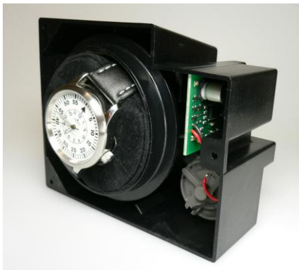
WTM front view with watch cushion and watch
